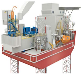
LIGHT WELL INTERVENTION CANTILEVER
